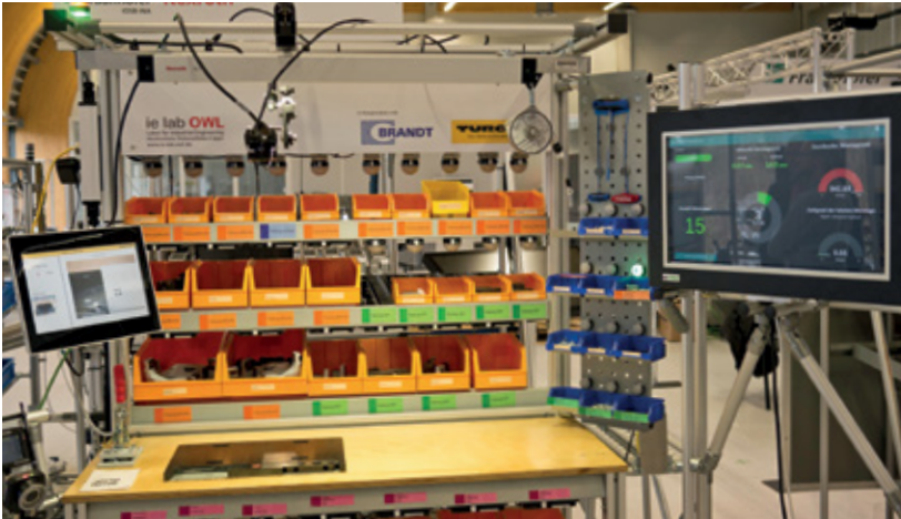
Continuous further development: The key indicator cockpit (right) was recently added to Turck's pick-to-light system
