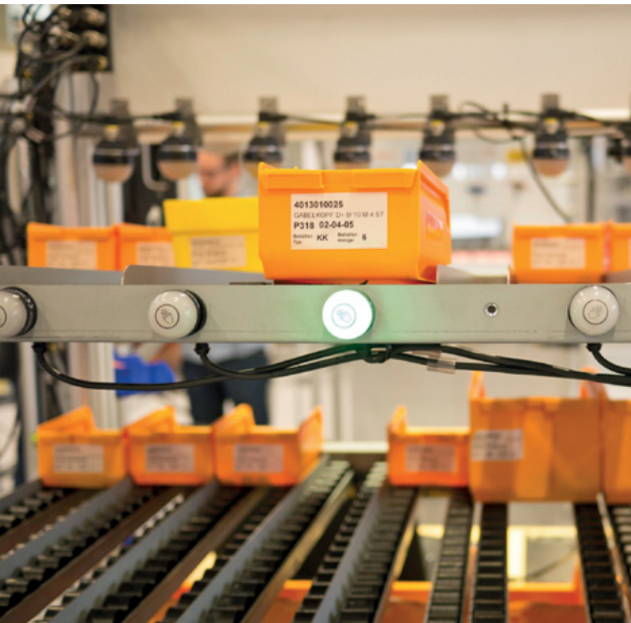
The put-to-light system indicates the row in which the newly filled container has to be inserted
