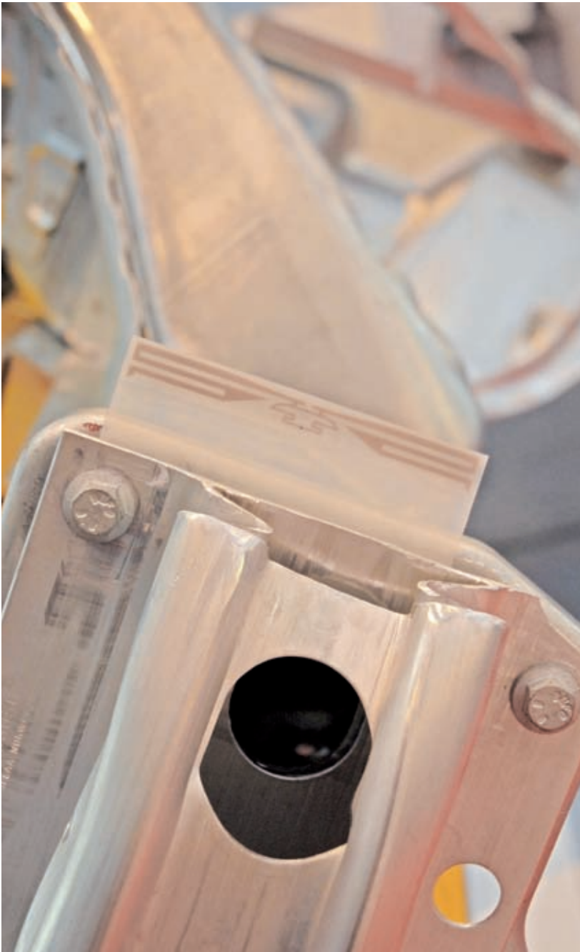
At Volvo in Gent, a robust plastic tag is attached to the side member of the vehicle body directly at the beginning of the shelling
