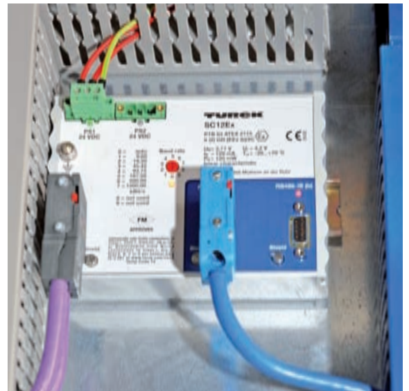
The SC12Ex segment coupler is used for intrinsically safe separation of RS485 and RS485-IS
