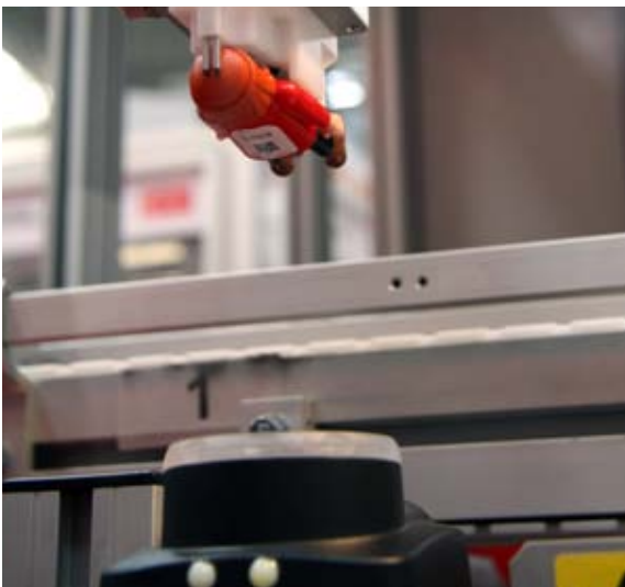
The DataMatrix/Barcode reader from the iVu family reads the code from the back of the figure
