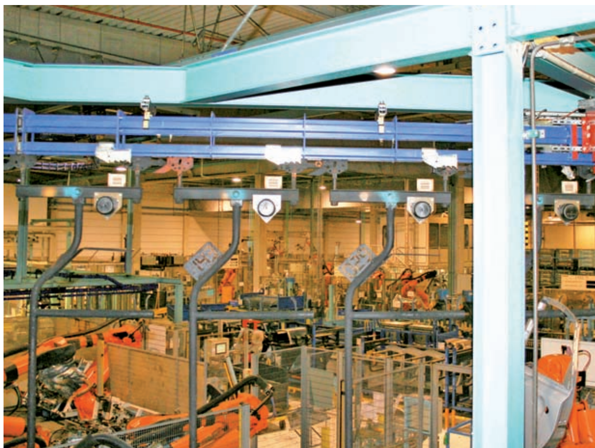
Until today, usually the transport systems are identified by RFID data carriers, like in this example the transport hangers of the supplier Tower Automotive
