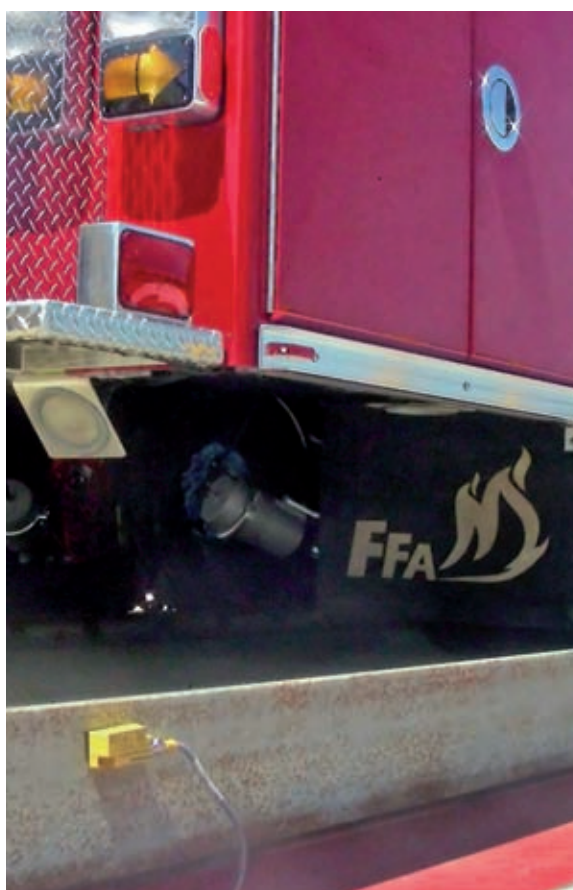
Turck inclinometers detect the angle of a tilt table
