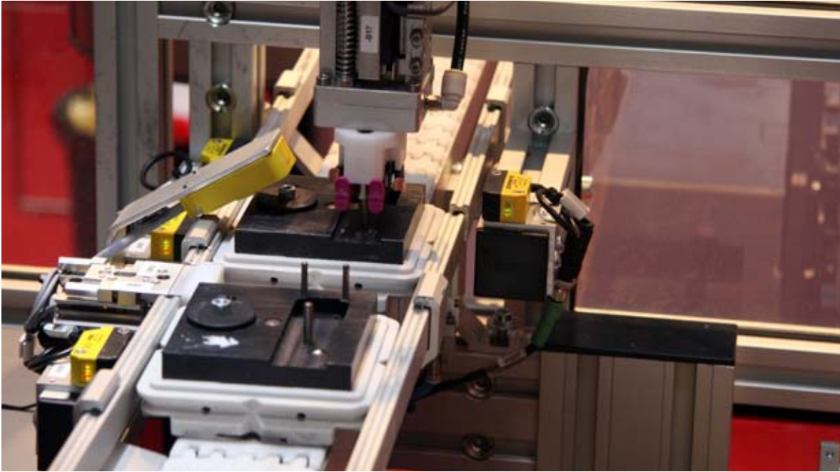
At the entrance of cell number 1, the BL ident RFID System from Turck reads the RFID tag on the workpiece
