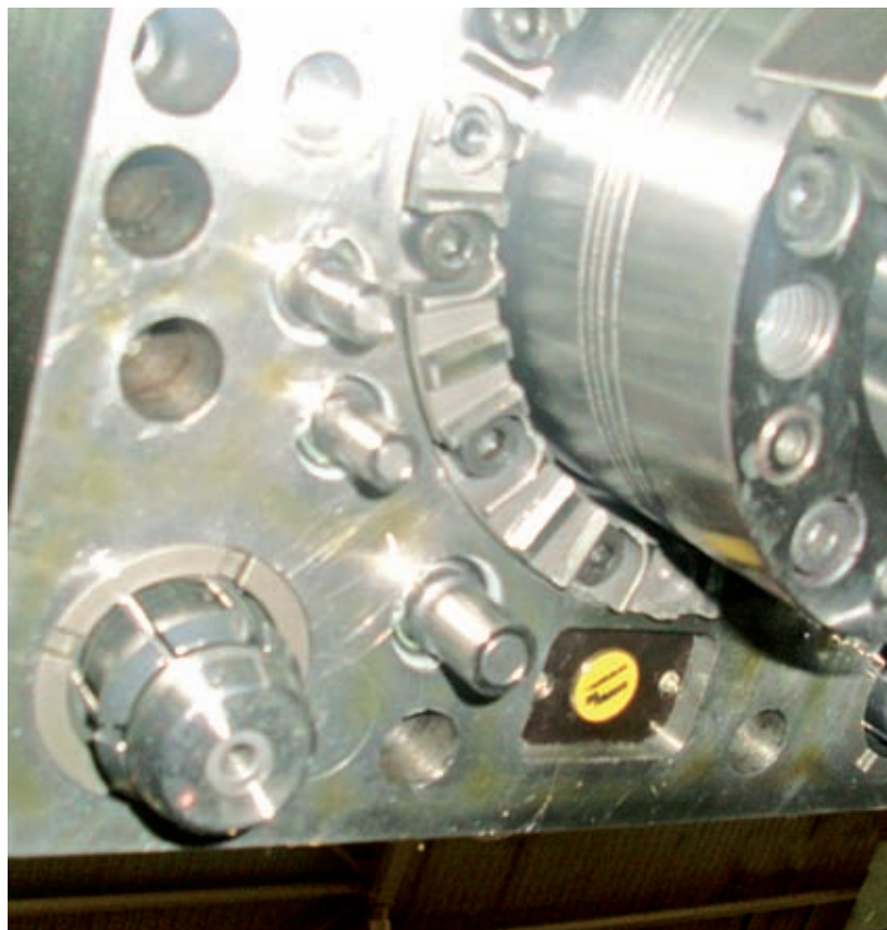
The robust read/write head on the machine reads the RFID tag on the cutting tool as soon as it is inserted
