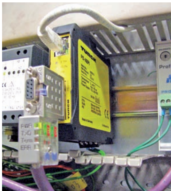
Ethernet-Interface and webserver of the PB-XEPI allow a central monitoring of the Profibus network
