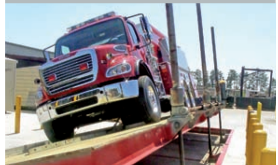
Ferrara Fire Apparatus Inc. in the USA guarantees the stability of their fire engines with a static tilting test – inclinometers from Turck measure the angle Page 40
