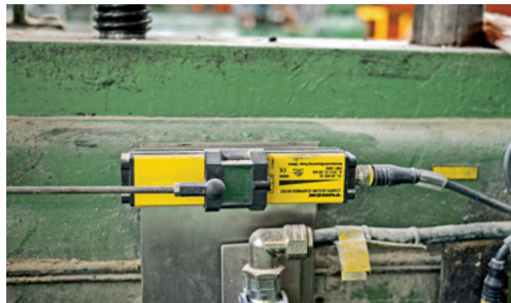
IO-Link linear position sensors measure the gap distance of rolling machines despite dust-laden environments and EMI
