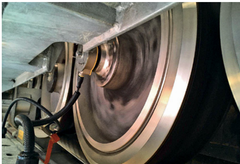
The QR24 encoder counts the rotations of the grooved rollers and sends the values to a higher level controller
