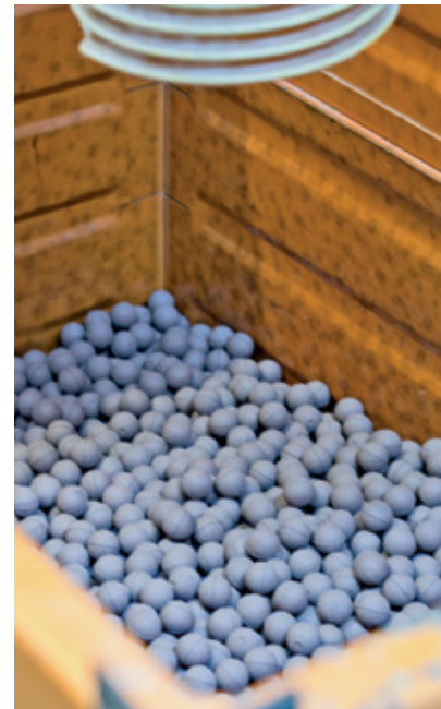
The cleaning balls made from natural rubber vary in design according to their intended application: They range in diameter from 14 to 48 millimeters
