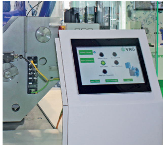
The TBEN-L I/O module and the TX513 HMI control and visualize the processes of the HYsec
