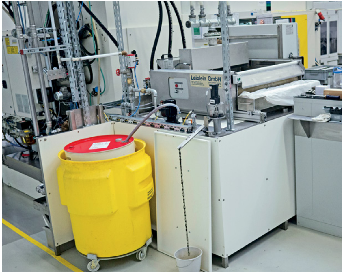
The barrel containing Robsol, RobMation's proprietary KSS coolant concentrate, is positioned at the back of the processing plant
